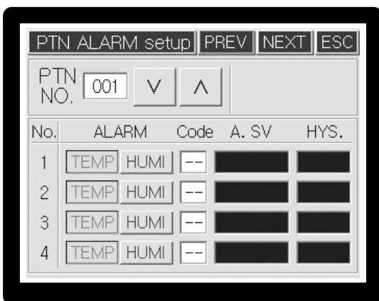
[FIG.59] Pattern alarm setup screen
