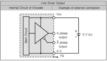
\*\* The output circuit of A, B, Z Phase (Line drive output A,  $\overline{A}$ , B,  $\overline{B}$ , Z,  $\overline{Z}$  Phase) is same,
