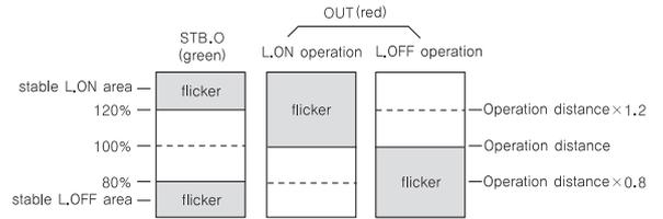
When using the selecting switch as L,ON, the red LED will be lighted once the light is turned ON. When using the selecting switch as D,ON, the red LED will be lighted once the light is turned OFF.
